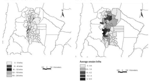
Figure 6. Annual erosion (tn/ha) - Western zone. Figure 7. Average erosion for each department - Present Present scenario. Current soil
