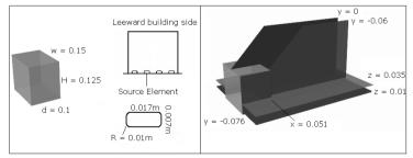
Figure 1: Building configuration and location of measurement planes
