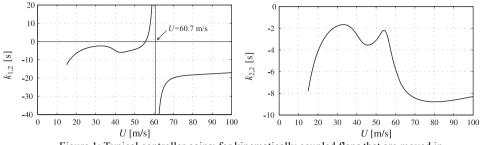
Figure 1: Typical controller gains; for kinematically coupled flaps that are moved in the same direction on the left, for separately driven flaps on the right.
