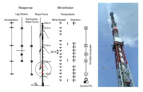
Figure 32: Wind and mast measurement equipment in Gartow
