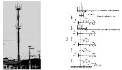
Figure 1: the mobile phone antennas support pole (centimetres).
