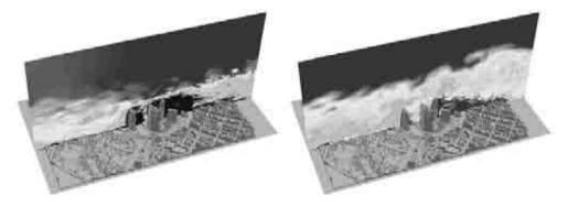
Figure 2: Instantaneous streamwise velocity and temperature field in the roughness layers over the actual city.
