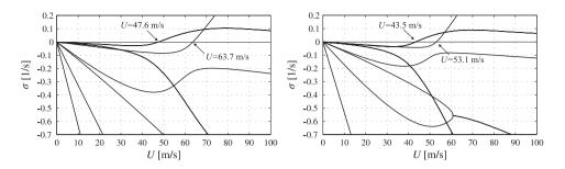
Figure 2: Real part  $\sigma$  of the system eigenvalues against the mean horizontal wind speed U. For a flap-free system on the left, for a system extended with unmoved flaps on the right.
