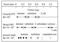
Figure 2: Shape of vortices and swirl ratio (with results by Church, 1979 and Monji, 1985)
