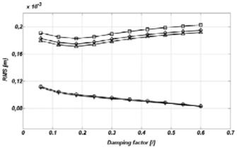
Figure 2: The RMS displacement of the top of the right tower as function of  $\zeta_{TMD}$  for various number of eigen-modes under consideration
