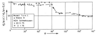
Figure 3: Rms. Pressure distribution at level z
