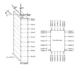
Figure 2: CAARC building model - HFPI pressure tap locations.
