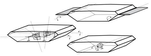
Figure 27: Actuators for stabilising bridges under wind action: aerodynamically effective control shields, twin control moment gyroscope and reaction wheel.
