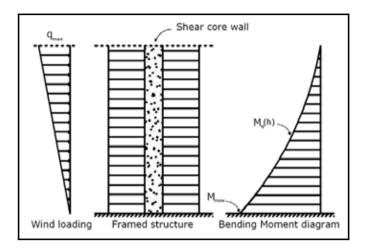
Figure 1: Structure with frames and shear core, under wind loading (left) and the bending moment diagram of the concrete core (right).
