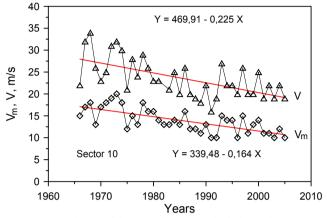
Figure 1. Many year change of the annual maxima of wind speed V (gusts) and V<sub>m</sub> (10 min mean) at the meteorological station in Wroclaw, sector 10 (central direction of the sector 10 is  $270^{0}$  - western).
