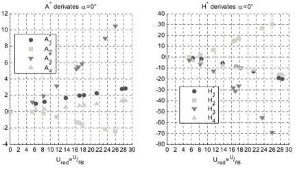
Figure 2: Flutter derivates at 0° angle of attack plotted versus reduced velocity.
