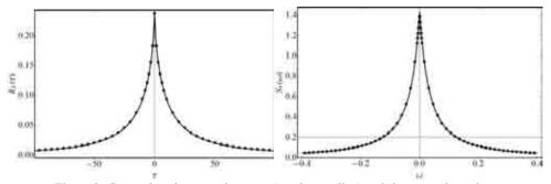
Figure 2: Comparison between the exact (continuous line) and the approximated (dotted line) Kaimal's correlation function (left panel) and PSD (right panel).
