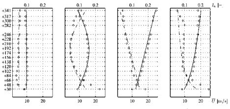
Figure 23: Typical wind profile classes at lower wind speed (o:  $\overline{u} \quad \Diamond: I_u$ )
