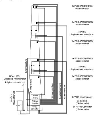
Figure 2: Overview of the planned measurement setup in natural scale
