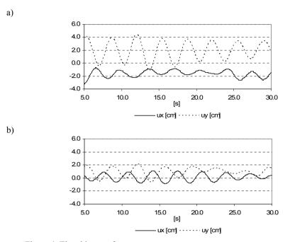
Figure 4: Time history of displacements-  $u_x$ ,  $u_y$  (comp. Fig.2b) -of the middle point of the top floor of the building: a) one building experimental situation- angle of wind attack equal to 135°, b) two buildings experimental situation- angle of wind attack equal to 135°.
