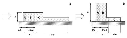
Figure 2: different pressure zones for buildings with non uniform heights (Fig. H.14 from CNR-DT 207/2008)
