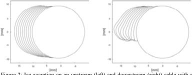
Figure 2: Ice accretion on an upstream (left) and downstream (right) cable with a cable spacing of 400mm. Icing conditions: wind velocity u=10 m/s, characteristic precipitation diameter MDV=75 $\mu$ m, air temperature T=-10°C, cable diameter d=349mm
