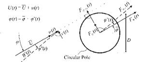
Figure 2: Wind velocities and forces on a circular cross section.
