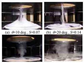
(c)  $\theta$ =60 deg., S=0.65 (d)  $\theta$ =70 deg., S=1.0 Figure 1: Flow visualization of tornado-like flow for various swirl ratios (without roughness block)
