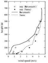
Figure 3: Mean velocity profiles at inlet.
