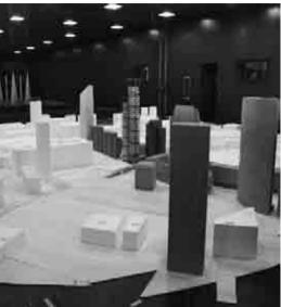
Figure 1: The model of the Tower in the Wind Tunnel, alone and with the surrounding.
