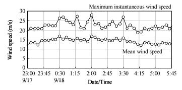
Figure 3: the mean wind speed and the maximum instantaneous wind speed for ten minutes in Typhoon No.12 in Japan
