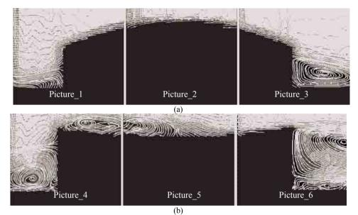
Figure 3: Wind tunnel tests: P.I.V. analysis.  $0^{\circ}$  (a) and  $90^{\circ}$  (b)Streamlines – three pictures for each wind direction angle
