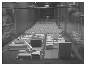
Figure 9: typical wind tunnel set-up for a pedestrian wind assessment study.
