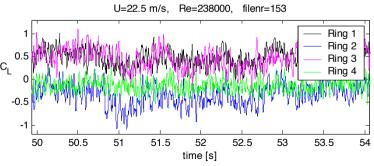
Figure 35: Time histories of lift coefficient at Re=238000, fixed cylinder inclined at 59.3° to the approaching flow
