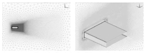
Figure 1: three-dimensional mesh used in the computations.
