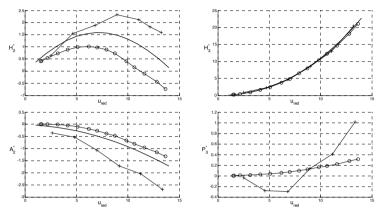
Figure 4: Examples of aeroelastic derivatives for a NACA 0020 airfoil ("-" Theodorsen's analytical solution, "+" free vibration measurement of Chowdhury and Sarkar (2003), "o" forced vibration measurement results)
