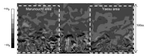
Figure 6: Instantaneous spanwise vorticity contour in mid section of the Marunouchi and Yaesu area.
