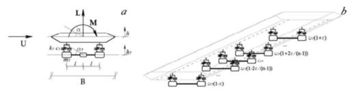
Figure 1: two-DOFs aeroelastic deck model equipped with two DOFs STMD device (a); sketch of the MTMD system.
