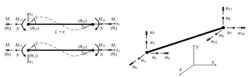
Figure 1. (a) Member basic displacements and forces (principal system); (b) Global reference system displacements.
