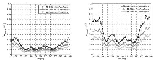
Figure 2: Point at the top-floor: peak-accelerations (3.5xRMS) in x and y direction in function of the exposure angle. Damping h=1%, 2%, 4%.
