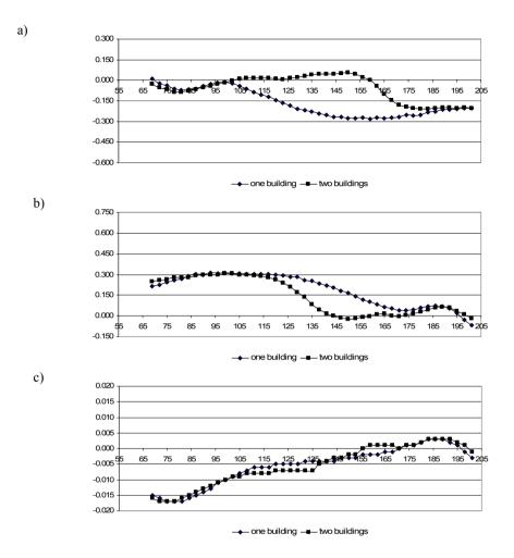
Figure 3: Functions of aerodynamic coefficients – a) drag coefficient  $C_x$ , b) lift coefficients  $C_y$ , c) moment coefficient  $C_m$  for the cross-section of the building on the level 134 m above ground (40<sup>th</sup> floor) in the two considered situations (one building and two buildings) obtained from wind tunnel tests.
