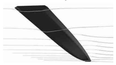
In Figure 5 the streamlines around the deformed bridge deck is shown.
