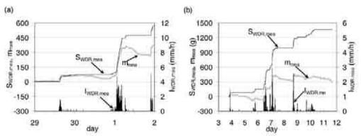
Figure 2: Measurement results of (a) November 29 - December 2, 2007 and (b) December 3 -12, 2007.  $m_{mea}$ : weight change of the specimen;  $S_{WDR,mea}$ : cumulative amount;  $I_{WDR,mea}$ : intensity of wind-driven rain.
