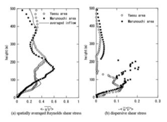
Figure 5: Spatially averaged Reynolds shear stress and dispersive shear stress profiles.
