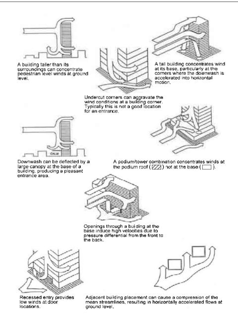
Figure 2: design features to change and/or ameliorate pedestrian wind conditions, after Cochran (2004).
