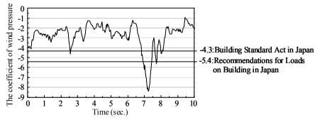
Figure 5: the coefficient of wind pressure for 10 minutes at P7 point
