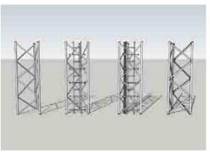
Figure 1: Lattice mast configurations used for full-scale section model testing. From left to right: 1A, 1B, 1C, 2A.
