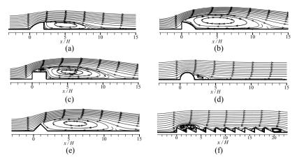
Figure 3: Streamlines distribution around the roofs of lower greenhouses
