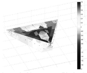
Figure 2: contour plot of the mean pressure coefficient for an incoming wind direction of 0 deg.
