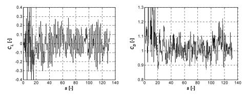
Figure 2: computed lift and drag coefficients ( $C_L$  and  $C_D$  are normalized respectively referring to the cylinder chord length B and height H).
