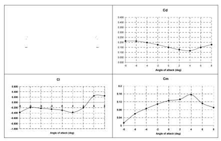
Figure 3: Aerodynamic coefficients for the preliminary design proposal.
