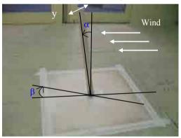
Figure 1: Orientation of square tower model
