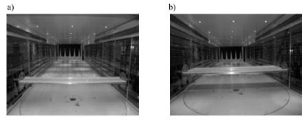
Figure 3: Sectional model of the deck in the wind tunnel working section: a) during tests of the windward deck, b) during tests of the leeward deck;
