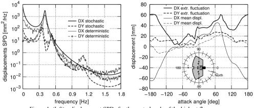
Figure 1: (left) – displacement SPDs for the central node of the highest floor, comparison between stochastic and deterministic analyses, angle of attack is 180°; (right) – extreme values of displacements fluctuations from the stochastic analysis, compared to static values.
