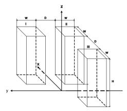
Fig.1 Schematic diagram of building models arrangement and coordinate system
