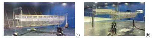
Figure 3: Sectional model in the wind tunnel: (a) test on a single deck (b) Wake effect tests.
