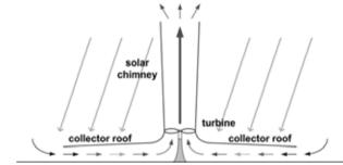
Figure 1: Building components of an SCPP: The central solar chimney and the collector roof
