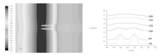
Figure 4: normalized x-velocity contours and velocity deficit - RSM
