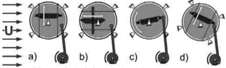
Figure 3: Degrees of freedom for forced vibration experiments
