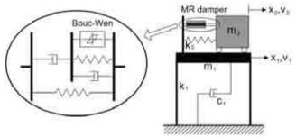
Figure 1: Smart TMD system using MR damper
