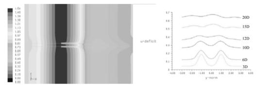
Figure 3: normalized x-velocity contours and velocity deficit - RNG k-E
