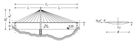
Figure1: Cable-stayed bridge under examination.
