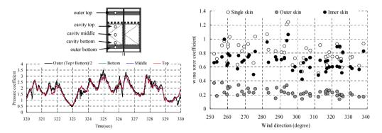
Fig.7 Pressure fluctuations on the cavity side of the inner skin.
