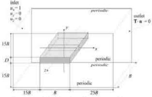
Figure 1: Analytical domain and boundary conditions
