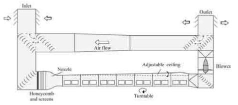
Figure 1: Low-speed boundary layer wind tunnel at the Institute of Aerodynamics, Technische Universität München
