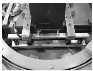
Figure 2: Detail of the suspension device. It is possible to see the elastic elements and the dampers.
