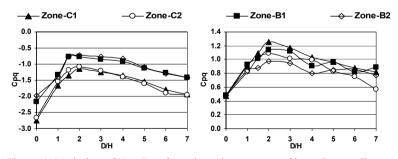
Figure 4. Variation of Net  $C_{pq}$  of overhang in presence of boundary-wall a) -  $C_{pq}$  b) +  $C_{pq}$
