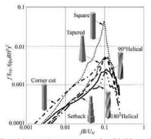
Figure 9: Crosswind overturning moment spectra for tall building models with various configurations (Tanaka et al., 2009)
