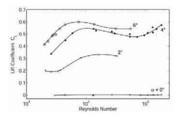
Figure 1: Lift coefficient upon the Reynolds number for different angles of incidence  $\alpha$
