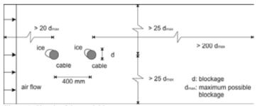
Figure 1: Sketch of the model layout
