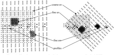
Figure 1: Obstacle arrangement and velocity measurement zones for the MUST wind tunnel case. Left: approach flow direction 0°. Right: approach flow direction -45°. Wind always from left.
