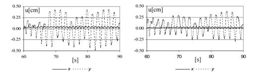
Figure 5: a) Displacements-  $u_x$  (horizontal),  $u_y$  (vertical)-of the middle point of the windward deck, b) displacements-  $u_x$  (horizontal),  $u_y$  (vertical)-of the middle point of the leeward deck.
