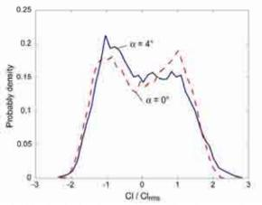
Figure 3: Probability density functions of lift fluctuations for two angles of incidence
