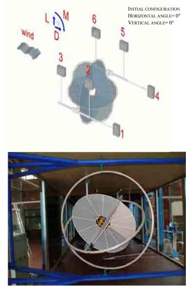
Figure 2: above: experimental setup (6 force measurement points) and sign convention; below: a view of the model in the CRIACIV wind tunnel
