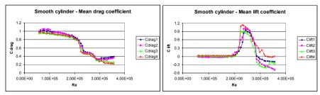
Figure 3: Mean drag and lift coefficients calculated by integration from the four pressure rings, denoted 1 to 4 from ground to ceiling, for a smooth surface cylinder.
