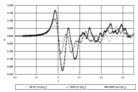
Figure 3: Variation of the transversal force acting on the plate N [N] with the time [s]. The legend indicates the angular rotation speed of the centrifuge arm. The plate is placed parallel to the motion direction.
