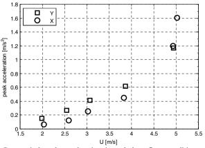
Figure 3: Cross wind peak acceleration in turbulent flow conditions. X: wind perpendicular to the long side of the rectangular section; Y: wind perpendicular to the short side.
