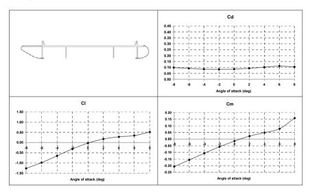
Figure 4: Aerodynamic coefficients for the modified design proposal.
