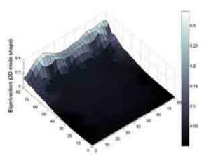
Figure 3: Referring to mode 1, wind direction angle equal to  $0^{\circ}$  and square plain structure (test p.2) – wind pressure fields processing with POD. technique: Eigen vectors three dimensional variation.
