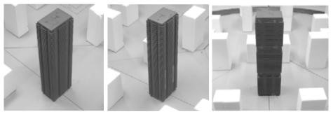
Figure 1: HFPI and HFFB models - CAARC building model with balconies.
