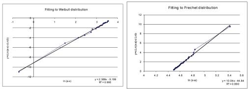
Figure 2.: Fitting of monthly maximum wind speed
