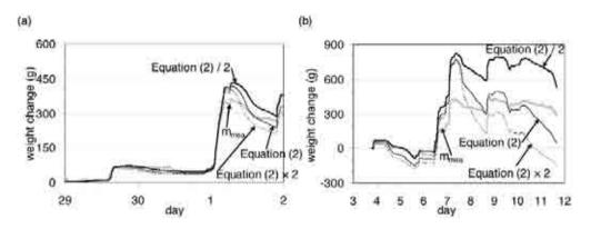
Figure 3: Simulated weight changes  $m_{sim}(I_{WDR,mea})$  of the specimen compared to measured ones  $m_{mea}$ . (a) 29/11/2007 - 2/12/2007 and (b) 3/12/2007 - 11/12/2007.
