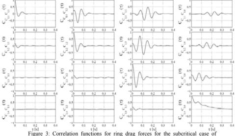
U=12m/sec. Propagation is evidently one-sided. Model setup,  $\varphi=60^{\circ}$  and  $\alpha=0^{\circ}$ .
