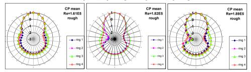
Figure 4: Mean pressure coefficients evolution with Re from the four pressure rings, denoted 1 to 4 from ground to ceiling, rough surface model.
