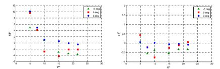
V\* for different mean angle of attack. (pedestrian deck, wind blowing from the sea).
