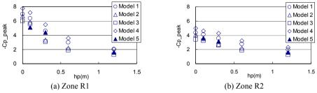
Figure 2: Effect of parapet height  $h_p$  and thickness  $t_p$  on  $C_{p_{paral}}$  in Zones R1 and R2.
