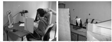
Figure 2: Experimental zone with an air duct on the right side of the subject, an infrared camera in front of the subject and a head position system in order to ensure a good impact area.
