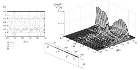
Figure 2: Pressure coefficient time histories and PSD along the upper side surface
