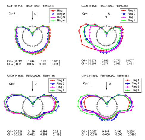
Figure 1: Mean pressure coefficients around cylinder at different Reynolds numbers, fixed cylinder inclined at 59.3° to the approaching flow
