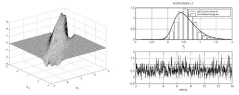
Figure 1: on the left, the function h(y) obtained for an order 3 autoregressive filter; on the right, above the target distribution with the histogram of a realization and below a window of the realization itself.
