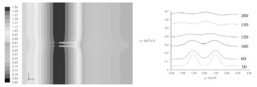
Figure 2: normalized x-velocity contours and velocity deficit - realizable k-e
