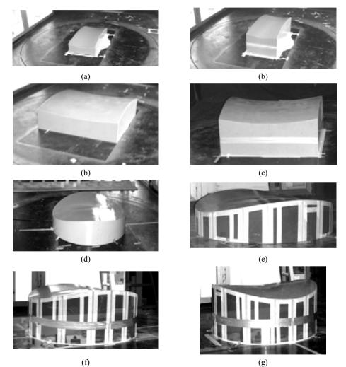
Figure 2: Wind tunnel tests: some of the different geometrical configurations tested. Rectangular (a, b) and square (c, d) models with two different geometrical configurations; Circular models (d, e, f, g) with two different geometrical configurations and two different types of roughness.
