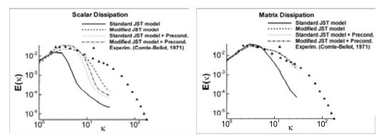
Figure 4: comparison against experiments of the spectrum of isotropic turbulence computed with several numerical approaches.
