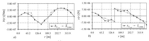
Figure 3: Diagrams of  $\bar{e}_{x,\max}(r)$  and of the load effects  $e_{Fx,eq}$  generated by the ESF  $F_{x,eq}(z)$  obtained using spectral eigenfunctions and imposing 14 conditions: a) e=b; b) e=s.
