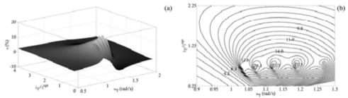
Figure 2: Control effectiveness of IMTDs ( $\varepsilon$ =0.15 and  $\delta$ =0.50) as a function of the damping ratio and of the frequency tuning: tridimensional view of the objective function  $\eta$  (a); contour plot of the objective function  $\eta$  in the region of the optimal solution (values in percentage) (b).
