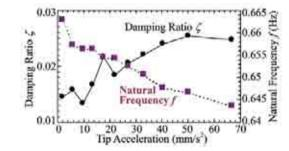
Figure 6: Variation of dynamic characteristics of a 99m-high steel-framed building (Tamura and Suganuma, 1996)
