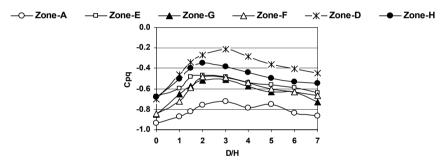
Figure 3. Variation of C<sub>pq</sub> on roof surface in presence of boundary-wall
