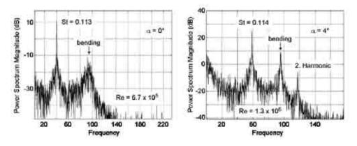
Figure 2: Power spectra of lift for rectangular section for two angles of incidence a
