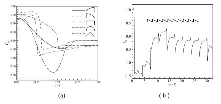
Figure 5: Variation of pressure coefficient C<sub>p</sub> with curve length ofperiodically placed roofs of lower greenhouses
