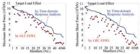
(a) Shear forces reproduced by GLF ESWL (b) Shear forces reproduced by LRC ESWL Figure 3: Comparisons of maximum shear forces reproduced by ESWL, GLF and LRC, and actual maximum shear forces obtained by dynamic time domain response analysis (Katsumura et al., 2007a)
