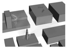
Figure 4: Stream traces for the flow field at the highest horizontal levels(the starting points for the stream traces, forward and backward, are along a diagonal line across the intersection directed from NW to SE at z = 150 mm; where the traces are not visible they are outside of the measurement domain 300 mm < x, y < 300 mm, 25 mm < z < 150 mm).
