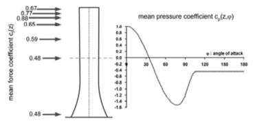
Figure 2: Distribution of wind force coefficients over the tower height
