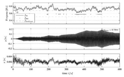
Figure 26: Time history of excitation frequency and corresponded deflection of the mast top
