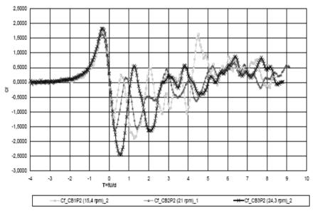
Figure 4: Variation of the transversal force coefficient  $C_f$  with the dimensionless time T = tU/d. The legend indicates the angular rotation speed of the centrifuge arm. The plate is placed parallel to the motion direction.
