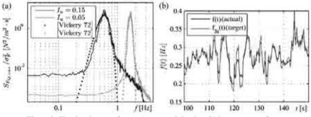
Figure 3: Simulated vortex forces: (a) spectral density, (b) instantaneous frequency.
