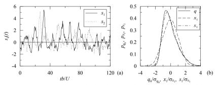
Figure 3: a – First two ICs; b – pdf of local pressure after a windward corner (solid line), pdf first PC (dashed line), pdf first IC (dash-dot line).
