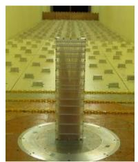
Figure 1: Pressure-tapped benchmark building model inside wind tunnel.
