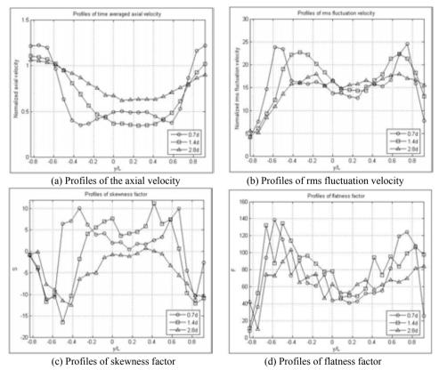
Figure 1: Variation of wake flow properties with the three downstream positions.
