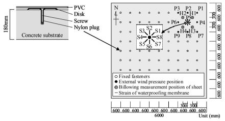
Figure 2: waterproofing membrane system and outline of the measurement
