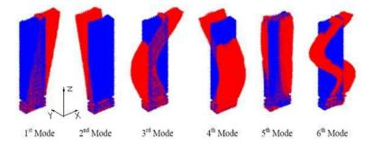
Figure 1: mode shapes of the finite element (FE) model of the tower with the coordinate system
