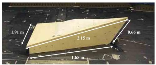
Figure 1: Geometry of the Cultural Centre (CC) building: 1:100 scaled model used for wind tunnel tests. Dimensions in model scale.
