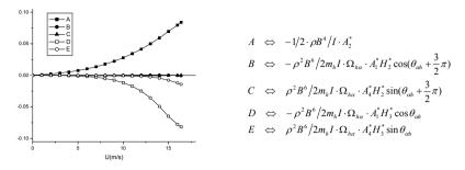
Figure 3: Aerodynamic damping of the systematic torsional motion
