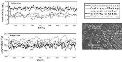
Figure 4: Time histories of the wind velocity and temperature in various local points at 65m height
