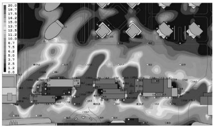
Figure 1. A comparison between a wind tunnel measurement and a CFD computation of the expected wind climate around a group of buildings.
