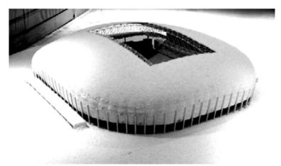
Figure 2: The stadium model covered with grinded Styrofoam ("artificial snow").
