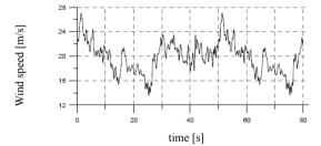
Figure 4: Exemplary wind speed (x component) simulated with WAWS method.
