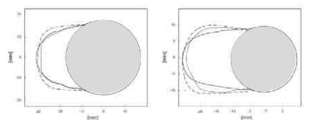
Figure 28: Ice accretion on single cables with different diameter
