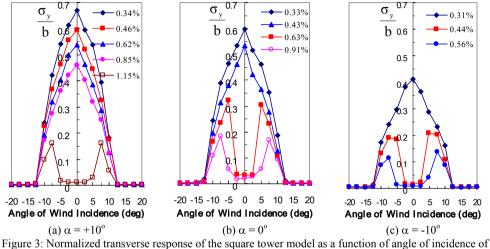
mean wind for various levels of structural damping
