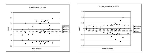
Figure 4: Differential pressures over both panels; negative values represent uplift loads; positive values represent forces directed to the roof.
