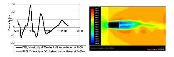
Figure 2: Time history of the Y velocity in the wake, comparison of DES and RNG k- $\epsilon$  model
