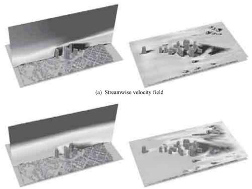
(b) Temperature field Figure 3: Time-averaged streamwise velocity field and temperature field in vertical section and horizontal section at 60m height.
