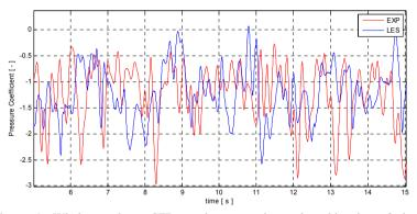
Figure 4: Wind tunnel vs CFD results comparison: time histories of the instantaneous values of the pressure coefficient.
