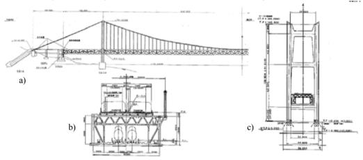
Figure 1: Bridge geometry (Courtesy of Dr. M. Nishitani HBSE-JP): (a) longitudinal profile, (b) deck section, (c) tower.
