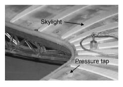
Figure 4: Model roof: skylights and pressure taps.
