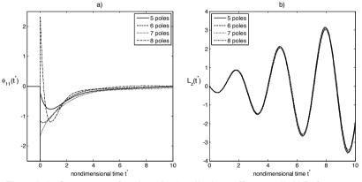
Figure 1: (a) Step response functions  $\Phi_{II}$  (amplitude cutoff at zero t\*) (b) Reference forces  $L_z$
