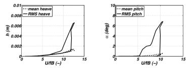
Figure 3: Heave (left) and pitch (right) amplitude rectangular deck characteristics as the functions of the wind velocity. The dashed line and solid line denotes the mean and root mean square value, respectively.
