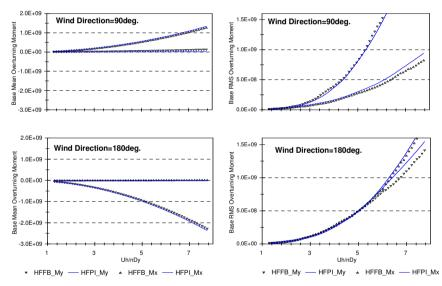
Figure 3: Comparison of base moments predicted by HFFB and HFPI methods as a function of reduced velocity
