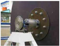
Figure 2 Turntable and force transducer configuration
