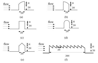
Figure 2: shapes of higher roofs and the computational zone
