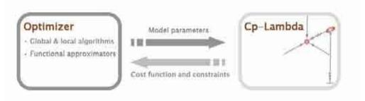
Figure 1: Coupling between optimizer and aero-servo-elastic solver for multi-disciplinary design optimization.
