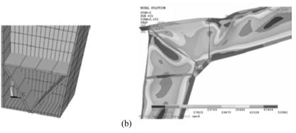
Figure 3: (a) Triangular stiffener at column support; (b) left haunch, von Mises stresses in psi (1 psi= 0.006895 MPa) (Duthinh et al., 2008).
