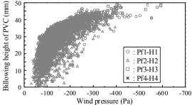
Figure 4: relationship between wind pressure and the billowing height of PVC
