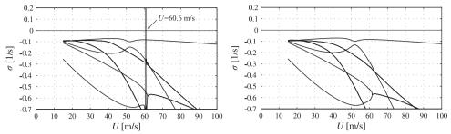
Figure 2: Eigenvalues of the aeroelastic system; controlled with kinematically coupled flaps that are moved in the same direction on the left, controlled with separately driven flaps on the right.
