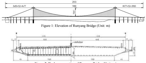
Figure 2: Deck cross-section of Runyang Bridge (Unit: m)
