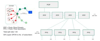
Figure 2: Open Fiber PON architecture
