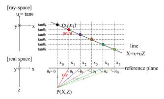
Fig. 6 "A group of rays through one point" in real space and corresponding points in orthogonal ray-space.
