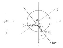
Fig. 10 Spherical ray-space expression of a ray.
