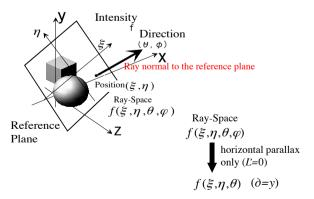
Fig. 3 Definition of spherical ray-space.
