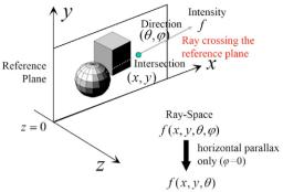
Fig. 1 Definition of orthogonal ray-space.
